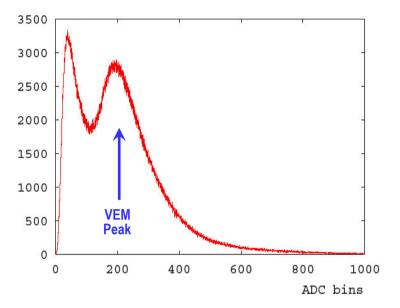
Detector calibration with the total charge deposited by the vertical muons crossing the center of the tank: VEM.
