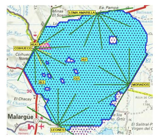
Surface Array 1600 detector stations 1.5 km spacing 3000 km<sup>2</sup> INFILL array: 60 detector stations 750 m and 433 m Spacing 100% duty cycle
