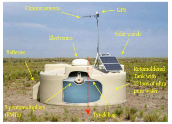
3.6 m diameter water tank containing a sealed liner with a reflective inner surface.
